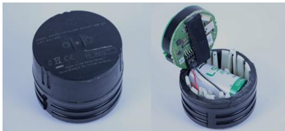
Fig. 9. Parking sensor closed (left) and open (right) [10]
