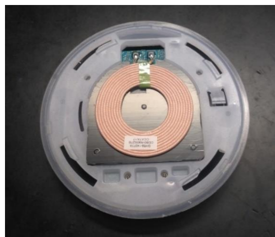
Fig. 3. Partially disassembled wireless charging pad, showing the copper induction coil and underlying PCB [6]
