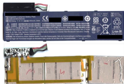
Fig. 1. Typical Li-ion-polymer notebook/tablet battery pack (top) and look inside the pack (bottom) [5]
